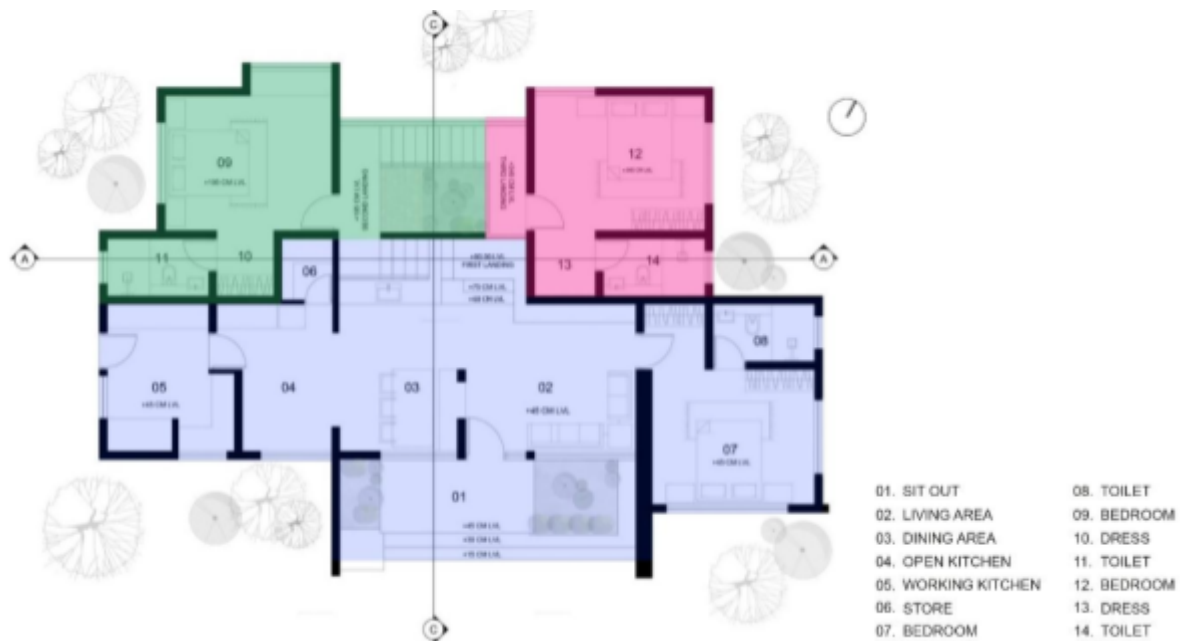
Fig. 9. Floor plan of Split-level residence (Each colour represents difference in floor height)(Akhil Albin Architects, n.d.)
