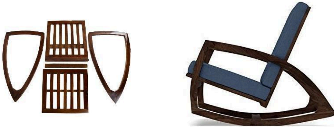
Fig. 6 An example showing a rocking chair traditionally a handicraft work converted to hybrid model where it is converted to modular parts and combined to make a unique piece that looks handmade but is modular.
